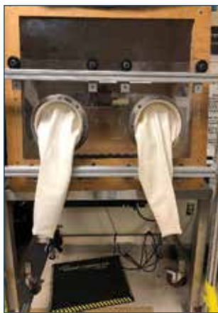
Figure 8 Set-up for the Dexterity Performance in Glovebox Shielding Study
